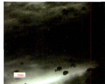
图3 内部具金属片及气泡 Fig.3 Metal sheet and air bubbles inside
